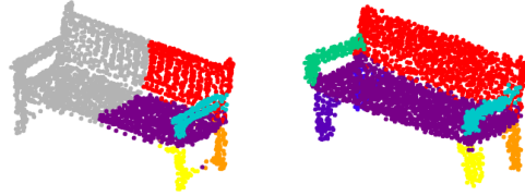
Figure 4: Shape completion. Left: Unseen data example with half of its variables obscured. Right: Shape completion using the ShapeVAE.
